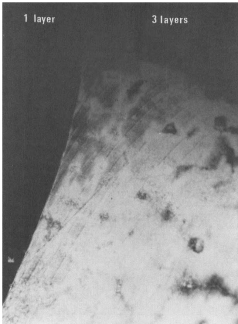
FIGURE 5 Monolayer to trilayer interface in cadmium arachidate showing "striations" in trilayer region.
